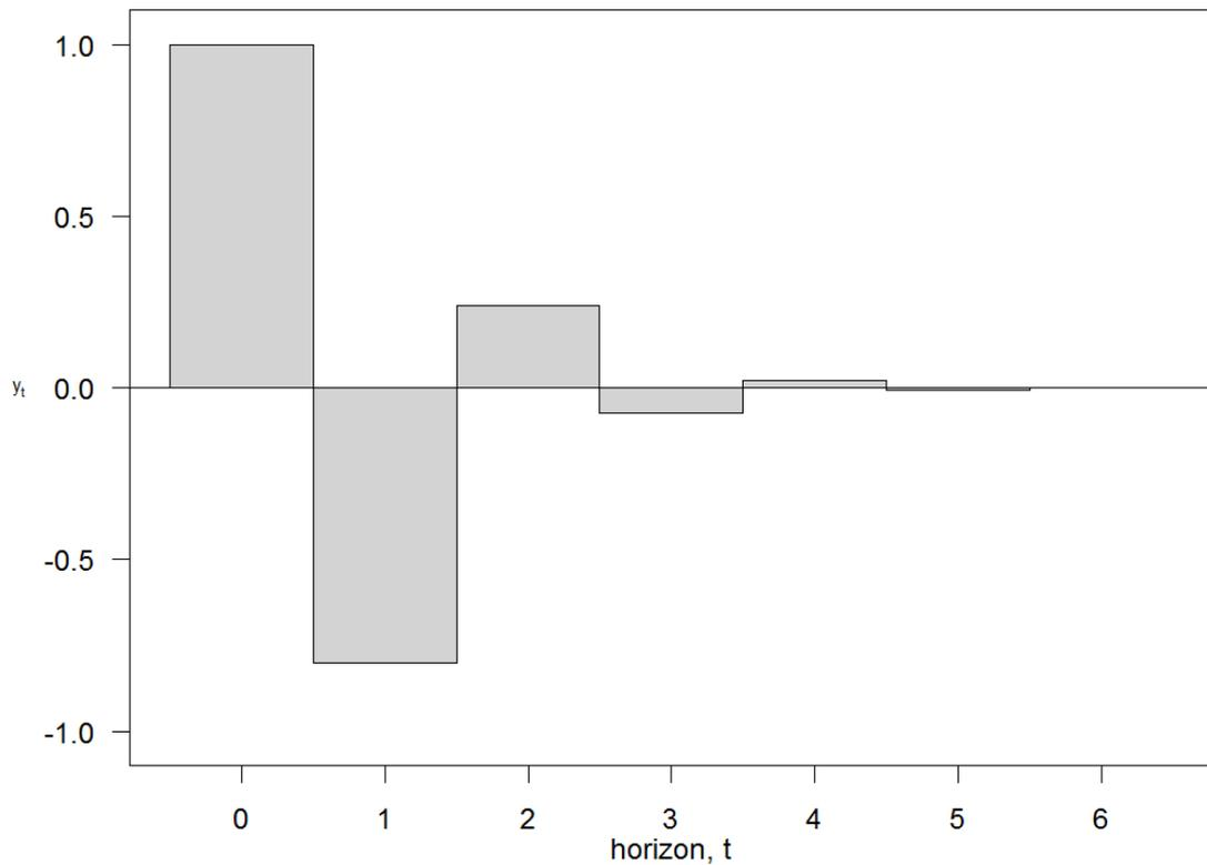
**Figure 1** – Example impulse response function for an ARMA(1,1) process,  $y_t = -0.3y_{t-1} + \varepsilon_t - 0.5\varepsilon_{t-1}$ . Here,  $\varepsilon_0 = 1$  and  $\varepsilon_t = 0 \forall t \neq 0$ . The impulse response function gives the effect of a unit shock on the dependent variable at different horizons.
